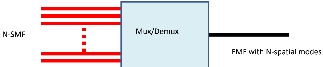
Schematic of photonic lantern in which N-input SMFs are coupled into the modes of an N-mode fiber.
