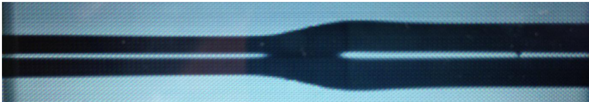
3-fiber photonic lantern on the left spliced into a graded index dual mode fiber to the right.
