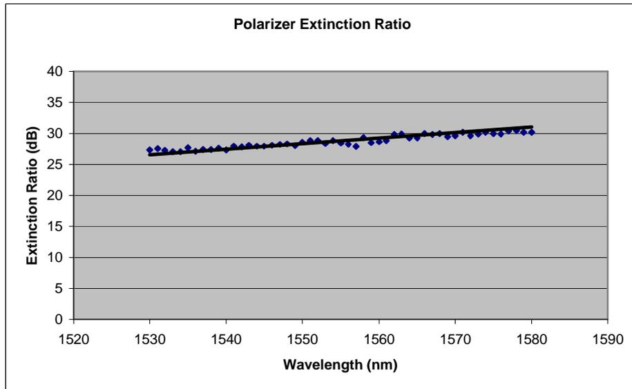
Phoenix engineers have modeled the evanescent field interaction and the graph below shows measured data (points) and data generated from the theoretical model (solid line) showing close correlation.
