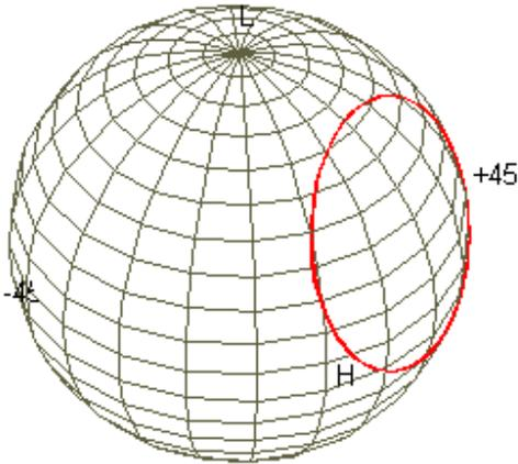
Changing the SOP after the waveplate can move the center of the described circle to any position on the sphere. A change in SOP can be caused by additional birefringent components in the fiber system following the waveplate or birefringence created in the output lead through tight bends or lateral force.
