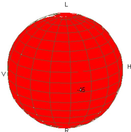
Applying a time varying current to the three sections provides continuous SOP scanning over the full surface of the Poincaré sphere.
