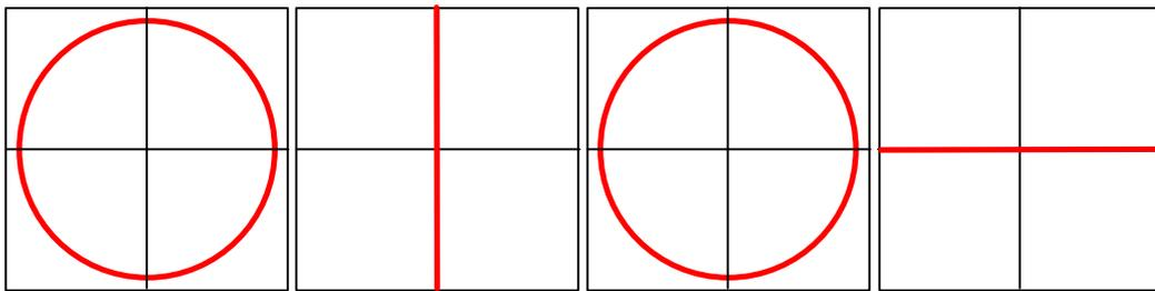
Change of linear output state, i.e. switching between the two axes, can be achieved by switching the drive current.
