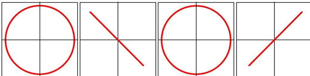
The SOP in the plane of the fiber tail output is dependent on the birefringence of the fiber tail and will be dependent on the temperature. However changes will be on the great circle around the sphere passing through both poles and the equator.
