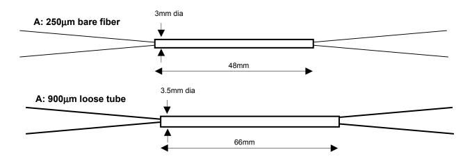
Package style B, rectangular cross section plastic package with throughput fibres.
